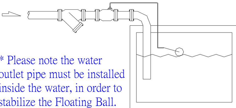
\* Please note the water outlet pipe must be installed inside the water, in order to stabilize the Floating Ball.
